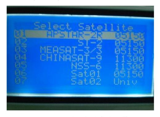
1. Press UP or DOWN to select the desired satellite, press OK to show transponder frequency contained in this satellite.(As below)
