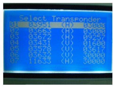
2. Press UP or DOWN to select the desired frequency, press LEFT or RIGHT to turn page, press OK to show the satellite name, frequency, signal intensity and quality, (As below)
