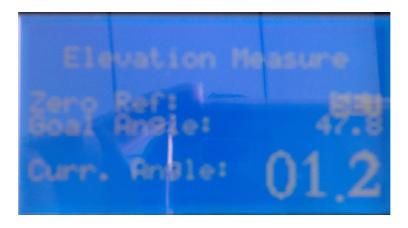
Zero Ref: If the current angle reading is not zero when place the unit to horizontal, press OK on "SET" to reset the angle.
