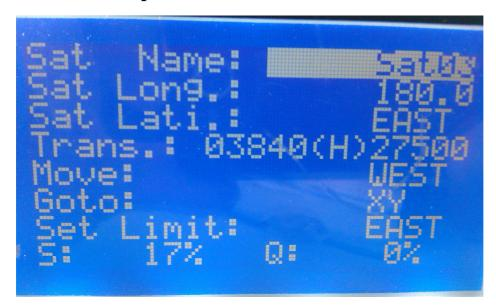
Sat.: Select a satellite (the satellite's USALS must be set to "ON")
