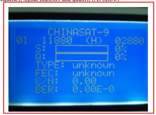
When the signal is locked, it will show current signal type, FEC, C/N and BER.
