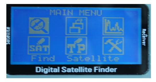
1. Press UP, DOWN, LEFT or RIGHT to select submenu, press OK to enter.
