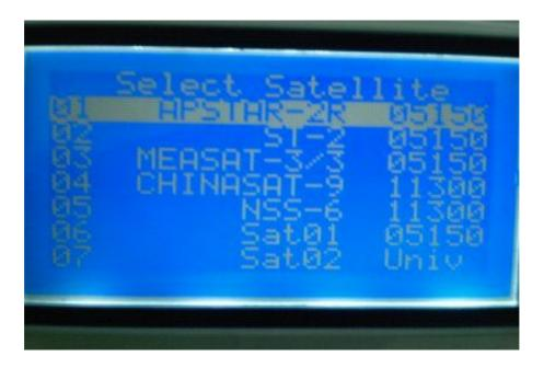
Use UP/DOWN/LEFT/RIGHT to move cursor to a satellite, then press OK to enter the transponder edit screen.
